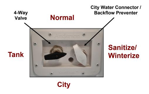
City – Pressure feed fixtures from 3/4" hose connection on backflow preventer.
